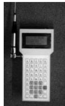
Fig. 4: Mobile TUBSAT-N communication terminal with integrated 12 channel GPS receiver.
